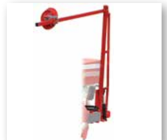
Hydraulic row marker up to 6 m
