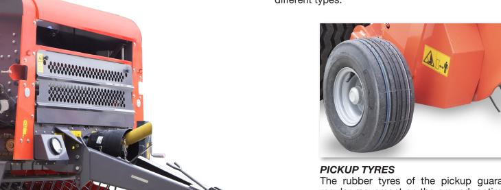
The rubber tyres of the pickup guarantee regular movement on the ground, optimizing and guaranteeing a clean collection of the product, for perfect storage and maintenance of nutritional properties.
