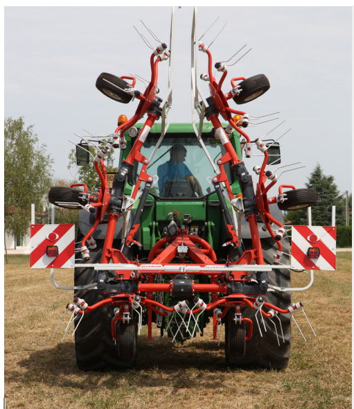
Cardan joint Easy access to greasing points. Ensures constant power to the rotors.
