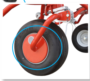
Wheels The wheels have a protective casing which prevents clogging.
