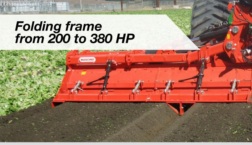
**JANE** is a bed tiller designed to meet the demands of medium-large farms. It is ideal for forming seedbeds for vegetable plants, both in greenhouses and in the open field. Depth is adjusted by means of a series of cylinders located on the rear of the bed forming hood, thus ensuring that the resulting shape and depth of the bed formed are constant during the pass.
