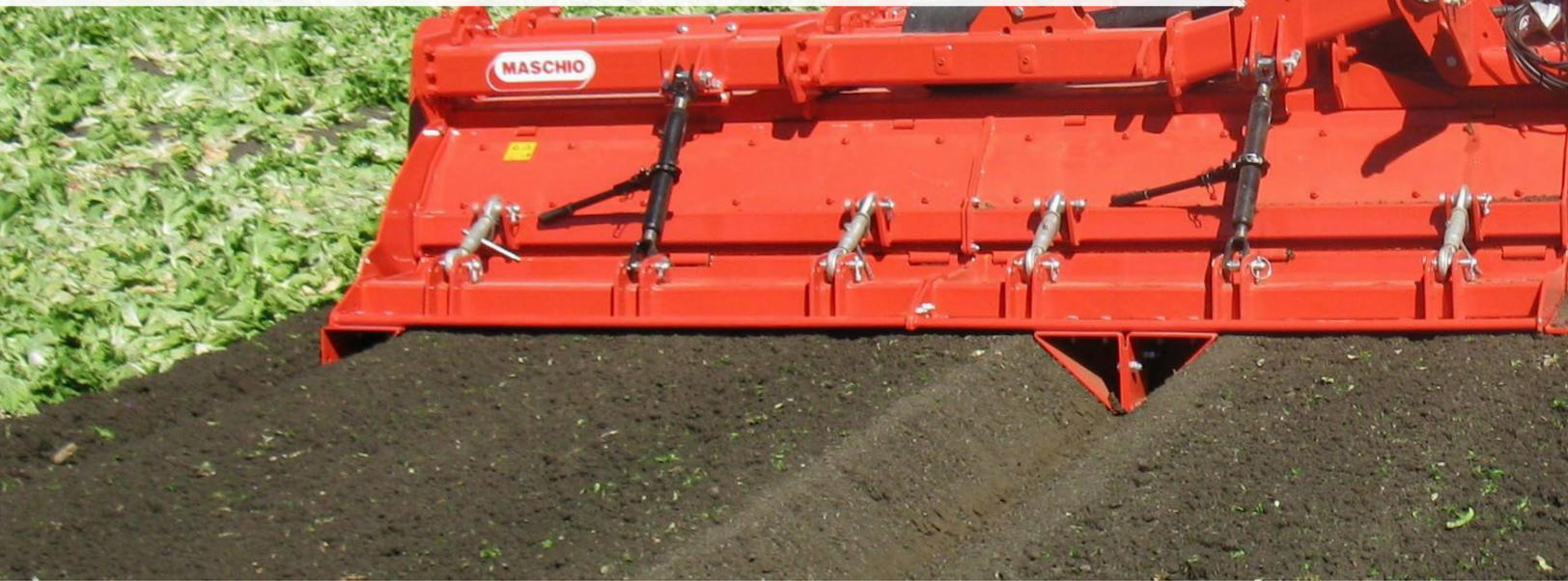
**JANE** is a bed tiller designed to meet the demands of medium-large farms. It is ideal for forming seedbeds for vegetable plants, both in greenhouses and in the open field. Depth is adjusted by means of a series of cylinders located on the rear of the bed forming hood, thus ensuring that the resulting shape and depth of the bed formed are constant during the pass.
