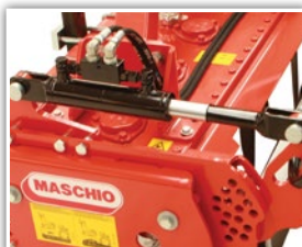
Hydraulic quick adjustment (OPT)
