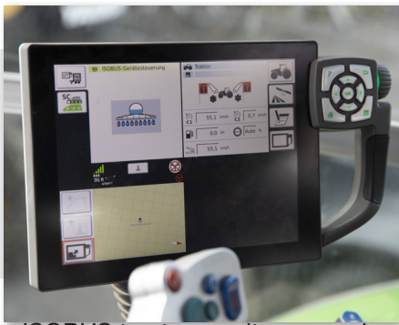
ISOBUS tractor monitor example
