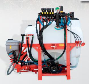
Farmers who need a reliable compact machine with many solutions of higher range will find the answer in **TEKO**. Available with **mechanical or hydraulic folding booms** and widths up to 18 m, this machine can be completed with many options like PRE-MIXER, complete self-cleaning system and tri-jet nozzles.
