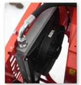
Hydraulic oil heat exchanger
