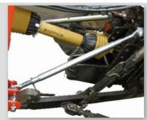
Pair of three-point hitch tie rods
