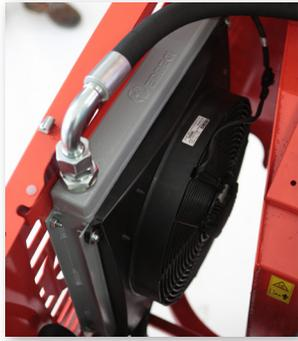
**Hydraulic oil heat exchanger**
