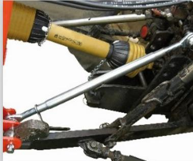
**Pair of three-point hitch tie rods**
