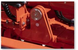
Used also for JUMBO, they ensure more robustness and resistance to contrast side wings' twisting.
